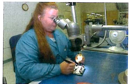
Tamara Burke solders surface mount parts on a circuit board at Synchron EMS in Melbourne. The manufacturing company received a grant to help them streamline their work processes. (Christina Stuart, FLORIDA TODAY)
